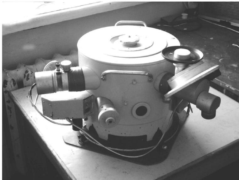
Figure 2. Spectrophotometer for water reflectance measurements (MHI RAS Marine Optics and Biophysics Department)
